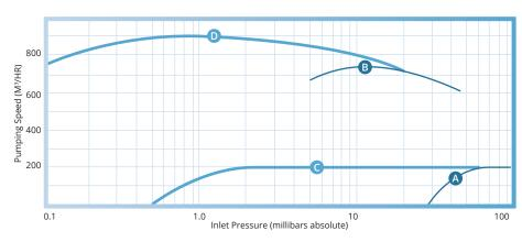
A: Performance of liquid ring backing pump B: Performance of booster pump HV1000 backed by liquid ring pump C: Performance of oil sealed type backing pump D: Performance of booster pump HV1000 backed by vane type pump
